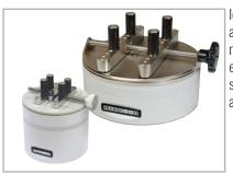
Ideal for testing torque on bottle caps and containers. Reversible jaws or movable posts, depending on model. effectively accommodate a variety of shapes and sizes. Capacities available from 10 ozFin to 100 lbFin.
