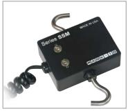
Measures tensile and compressive loads for a wide variety of applications, available in capacities from 0.25 lbF to 100 lbF. Threaded holes on two sides can accept a variety of hooks and implements, making this sensor particularly well suited for inline tests.
