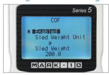
The COF is calculated based on the sled weight, adjustable from 100 to 1,000 g, to conform to various standards. A password can be set to protect settings from unauthorized changes.
