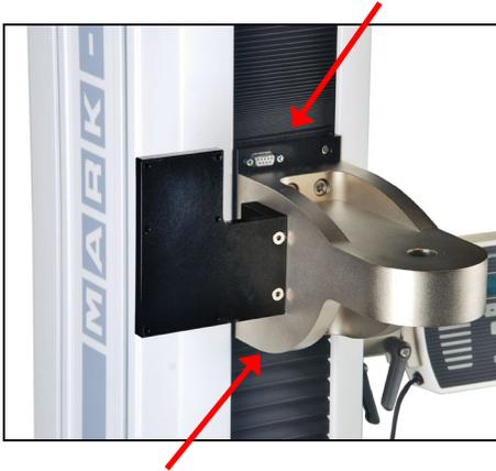
2. Using a brush, apply a small amount of general purpose bearing grease to the screw, as shown in the image below:
