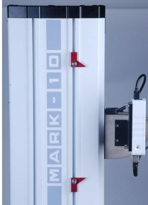
Limit switches allow the operator to set a location along the column at which point the crosshead will stop moving. Limit switches are located on the left side of the test stand column, as shown in the image to the left. Adjust their positions by loosening the thumb screws, repositioning, and re-tightening the thumb screws.
