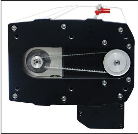
2. The drive belt must be removed. To do so, the motor mount screws must be loosened to permit the motor to be moved, reducing tension on the belt. Access to the motor is located in the back of the column. Remove the lower sheet metal cover to expose the motor and MDU. Then, remove the MDU. The motor will now be clearly accessible. Refer to the image below for locations of the motor mounting screws:
