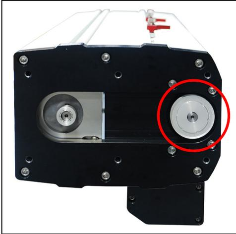
4. Remove the pulley from the ball screw, identified above, by loosening two set screws. The underside of the column now appears as follows:
