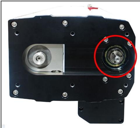
5. Apply grease to the bearing identified above in the same fashion as the upper bearing.
