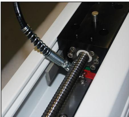
5. Cycle the crosshead up and down several times until the newly applied grease has been spread evenly over the length of the slide.
