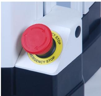
The Emergency Stop button is located on the base, adjacent to the lower right corner of the column, as shown in the image at left.
