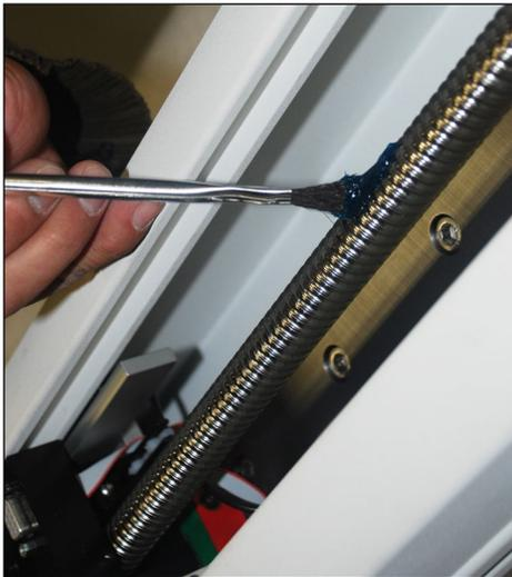
3. Cycle the crosshead up and down several times until the newly applied grease has been spread evenly over the length of the screw.
