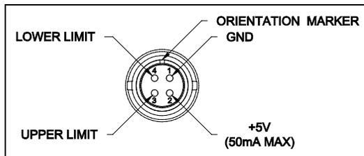
Note that when pins 3 and 4 are not connected, the auxiliary limits are inactive. When the +5V from pin 2 is connected to either pin 3 or pin 4, the respective limit becomes active and the crosshead is prevented from movement in that direction. The hard-wired cable and connector, as shown below, should remain in place if external limit switches are not used:
