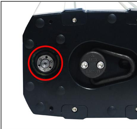
2. Apply general purpose bearing grease along the perimeter of the bearing. Wipe clean any excess grease.
