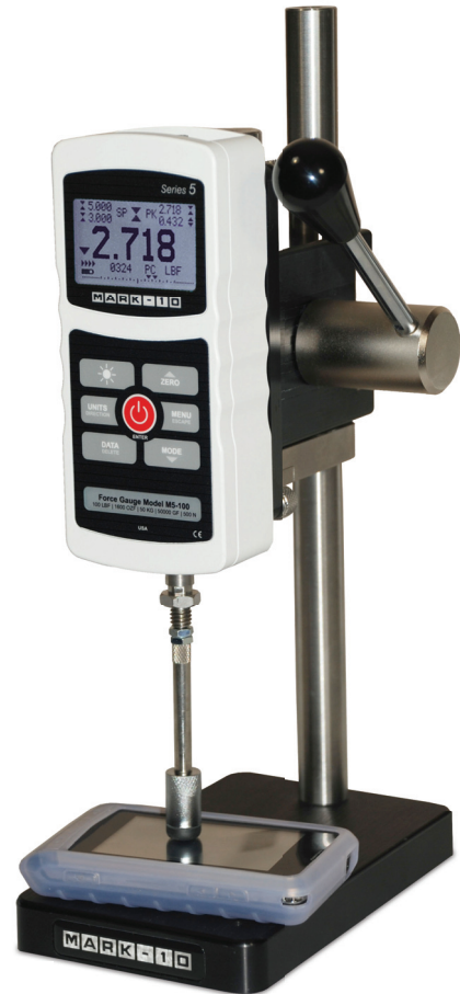
The ES05 is shown in a switch contact activation test, with Series 5 digital force gauge, extension rod and rubber tip attachment.
