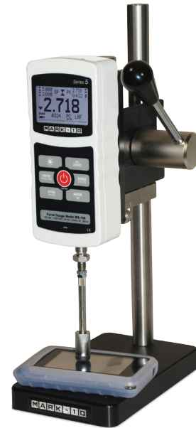
The ES05 is shown in a switch contact activation test, with Series 5 digital force gauge, extension rod and rubber tip attachment.
