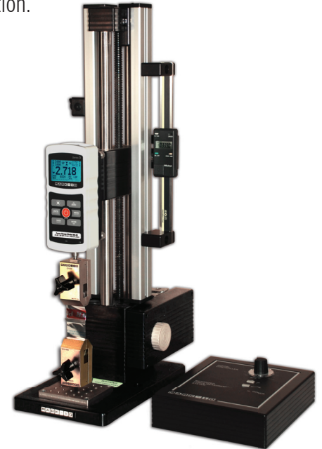
The ESM is shown in a typical tensile testing application, with Series 5 digital force gauge, digital travel display, limit switch kit, and wedge grips
