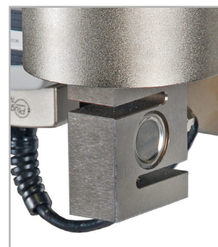
^ Series R01 sensor with shortened cable is shown mounted to an ESM1500LC test stand.*
