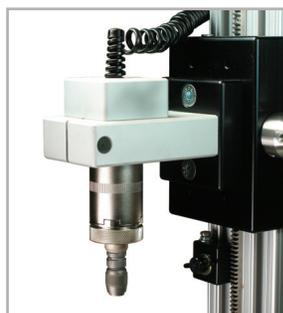
^ A Series R51 torque sensor is shown mounted to a model TSTM motorized torque test stand using optional AC1015 mounting kit.
