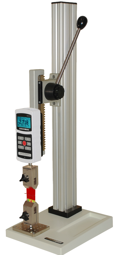
The TSB100 is shown with a Series 5 force gauge
