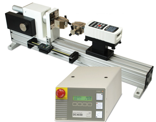
The TSFM500H-DC is shown configured for a tensile test, with Model M5-1000 digital force gauge and wedge grips.
