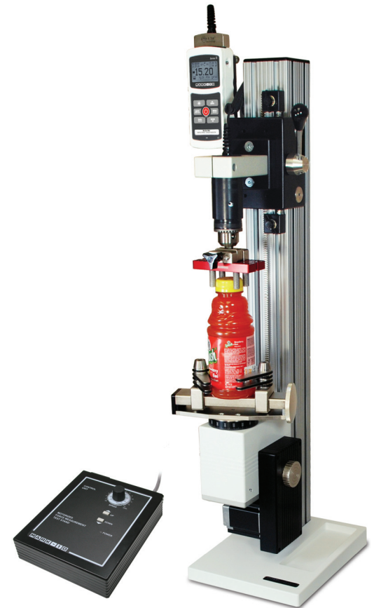
The TSTM is shown in a cap torque test, with a Series R50 torque sensor, Model M5i force/torque indicator, G1023 universal closure grip, and G1053 cap grip
