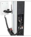
Connect the coiled cable to the connector marked CONTROL PANEL on the back of the test frame.
