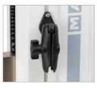
The mounting arm is pre-installed into the front right slot in the test frame column via two screws. Loosen the knob sufficiently to slide the ball, mounted to the rear of the tablet, into the arm. Adjust the viewing angle as desired, then tighten the knob.
