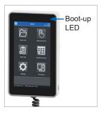
After turning on power to the test frame, the control panel will start booting up. An LED in the upper right corner will flash until the welcome screen appears.
