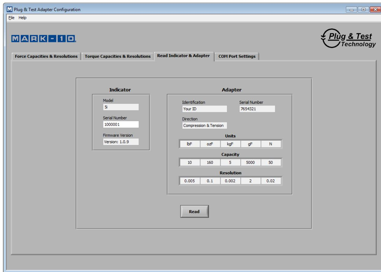
Use this screen to view information about the sensor and indicator. Click **Read** to view the indicator model number, serial number, and firmware version. The sensor's identification number, serial number, direction(s), capacities, and resolutions are also visible.
