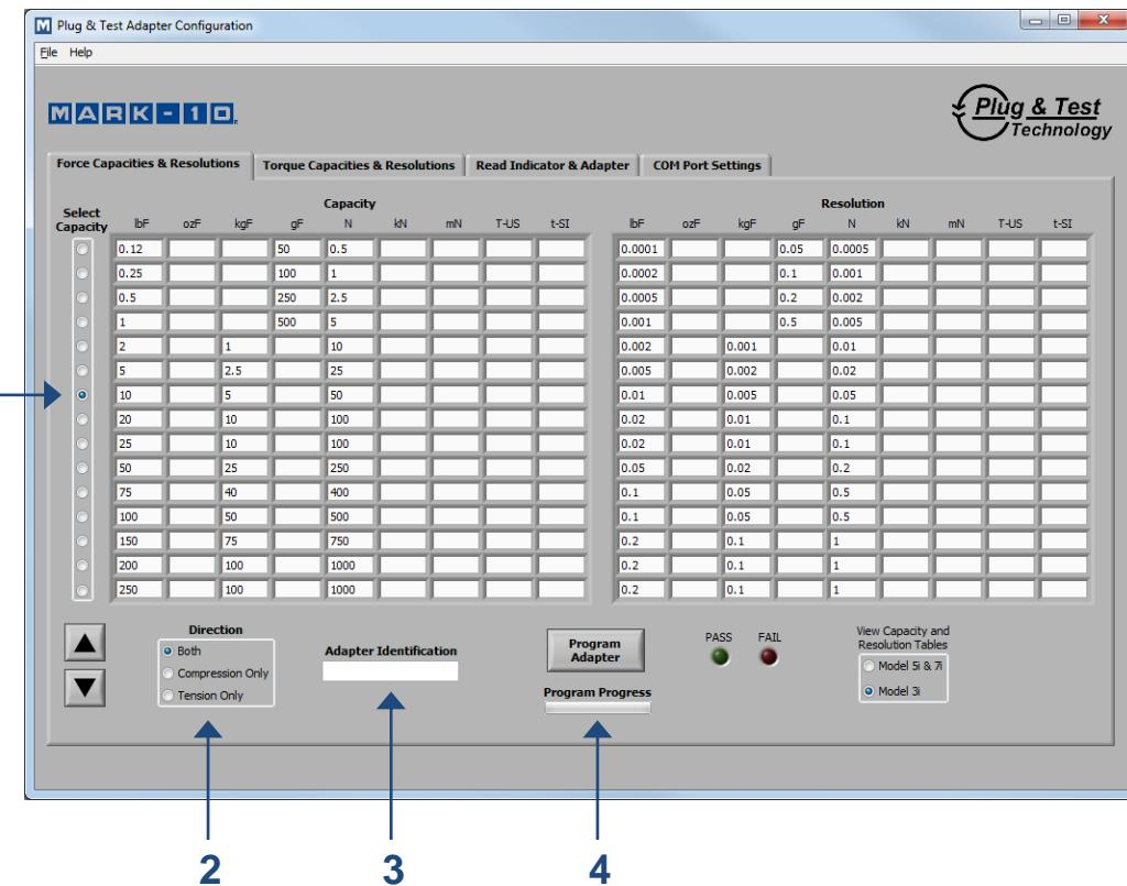
Use the **Force Capacities & Resolutions** and **Torque Capacities & Resolutions** screens to program the capacity appropriate for the sensor. The number of available units of measurement and displayed resolution depend on the indicator being used. Refer to Section 5 for detailed information.
