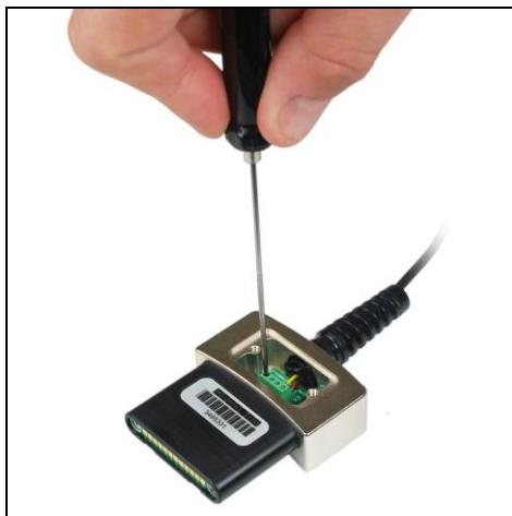
4. Install the strain relief by pressing it into the receptacle in the PTA housing, as illustrated below:
